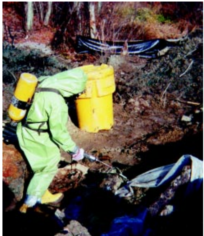
Air Monitoring being conducted in level B protection for locating and excavating contamination
